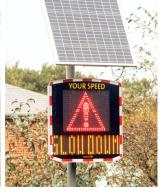
You may well have noticed that the Parish Council has installed new vehicle speed warning signs in the village. They're more sophisticated than the earlier devices, and can be programmed to display, in different colours, the speed vehicles are travelling. They have solar panels to charge their batteries, allowing them to operate for longer.
